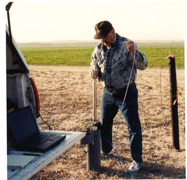
Retired UNL technician Jerry Leach installs digital water level monitoring equipment in a monitoring well.
