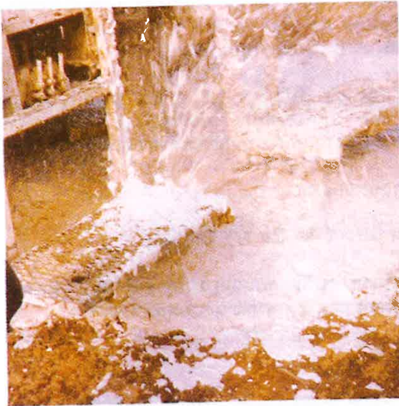
Figure 11.34. The liquid-volume fraction determines how the foam looks as it leaves the borehole. If the foam is relatively dry, it collects around the top of the borehole (left). If the LV tends to run away on the surface of the water brought up the borehole. ( Nelson Well Service Company )
