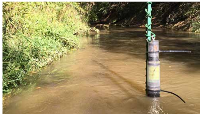
Multi-parameter meter deployed to measure 24 hour dissolved oxygen variation at Antelope Creek, Cedar County.
