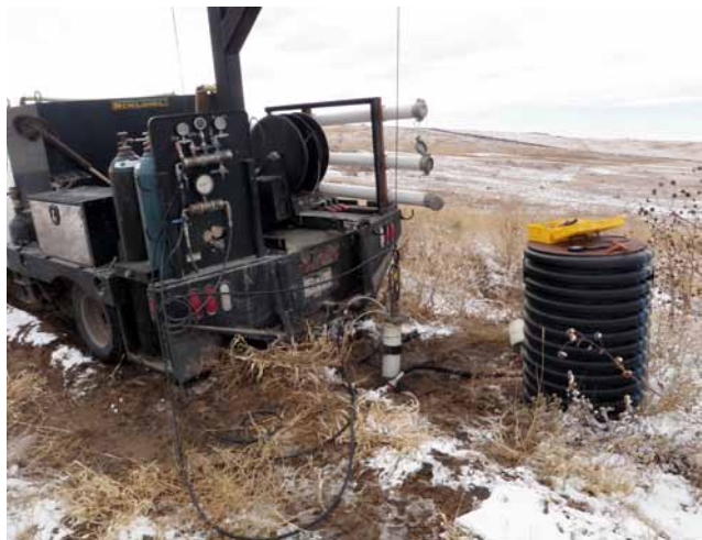
Mechanical integrity test at Crow Butte Resources Inc., Dawes County.
