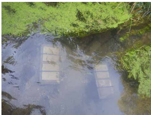
Benthic algae sampler used to collect benthic chlorophyll and algal composition data at Antelope Creek, Cedar County.
