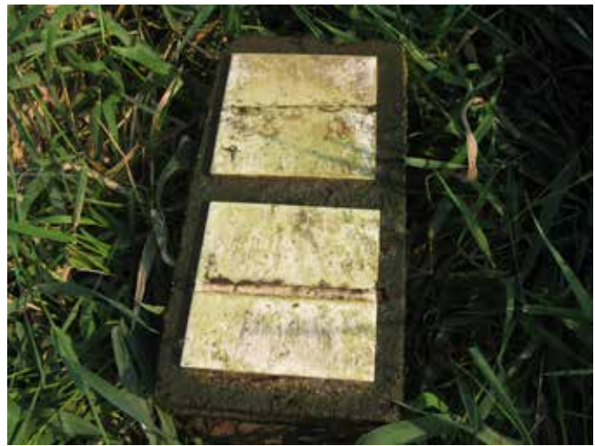
Benthic algae sampler upon removal from a stream after a three week deployment.
