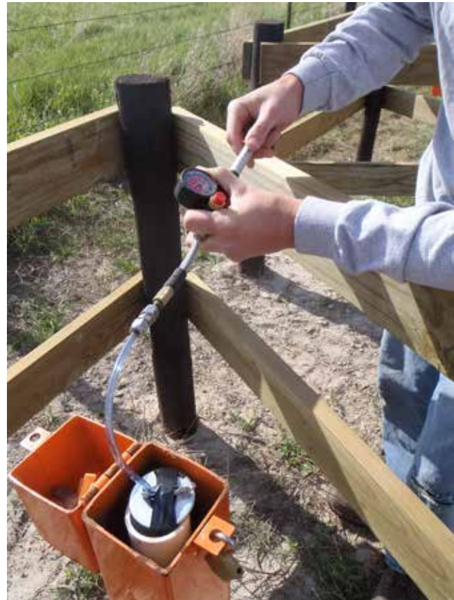
Sampling a dedicated monitoring well in the Lower Loup Natural Resources District.
