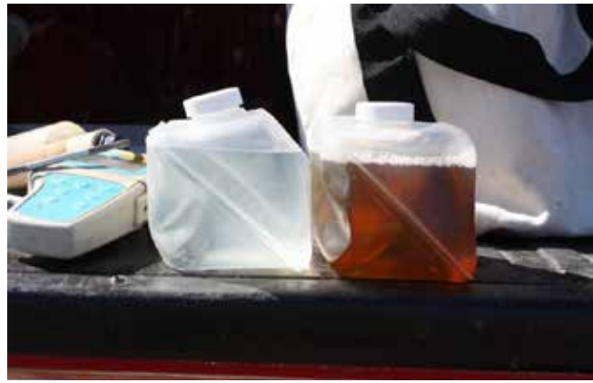
Samples from groundwater monitoring wells near a lagoon.
