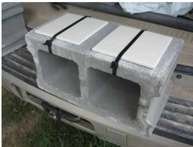
Benthic algae sampler constructed of two 6"x6" ceramic tiles zip-tied to a concrete block.
