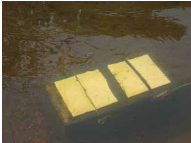
Benthic algae sampler used to collect benthic chlorophyll and algal composition data, Lost Creek, Colfax County.
