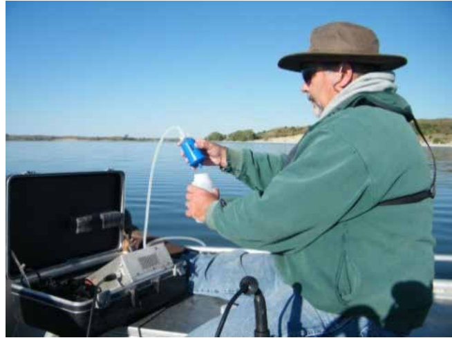
Filtering water for a chlorophyll sample at Merritt Reservoir, Cherry County.
