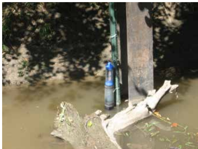
Multi-parameter meter to measure 24 hour dissolved oxygen variation, Loseke Creek, Platte County.
