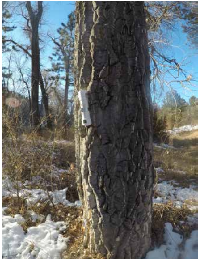
Air pressure sensor used to compensate instream pressure sensors to measure stream depth/stage.
