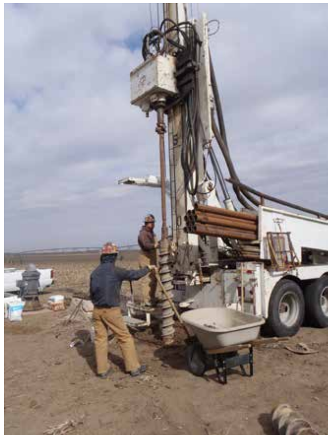
Drill rig collecting a vadose zone soil core in corn field, Clay County.
