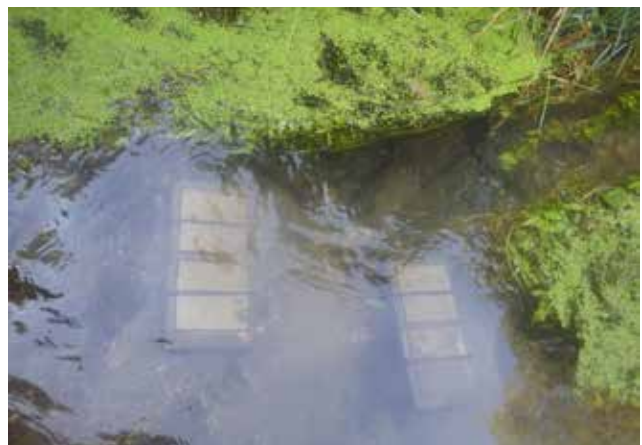
Benthic algae tiles used to collect benthic chlorophyll and algal composition data at Antelope Creek, Cedar County.
