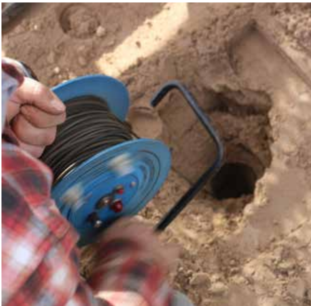
Measuring water table depth in a borehole after extracting core. Source: https://nebraskavadose.unl.edu
