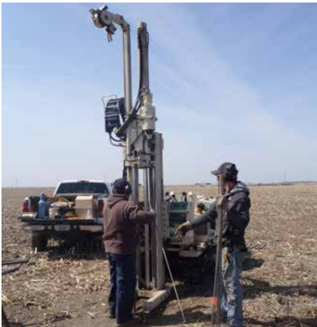
Geoprobe collecting a vadose zone soil core, Clay County.
