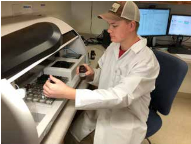
Preparing samples for microcystin analysis in NDEEs new microtiter plate format analyzer utilizing ELISA assays.
