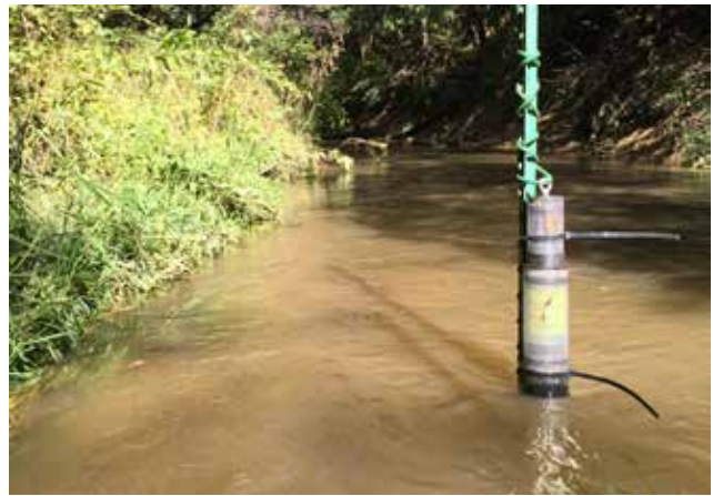
Multi-parameter meter deployed to measure 24 hour dissolved oxygen variation at Antelope Creek, Cedar County.
