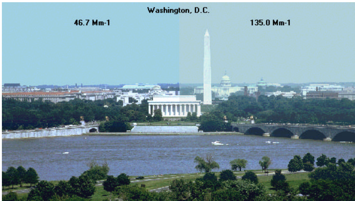
Fig. 2-4. Visual quality of scene from Washington, D.C. skyline. Left scene is visual quality under natural background conditions. Right scene is visual quality under average of the 20% worst days at this site.
