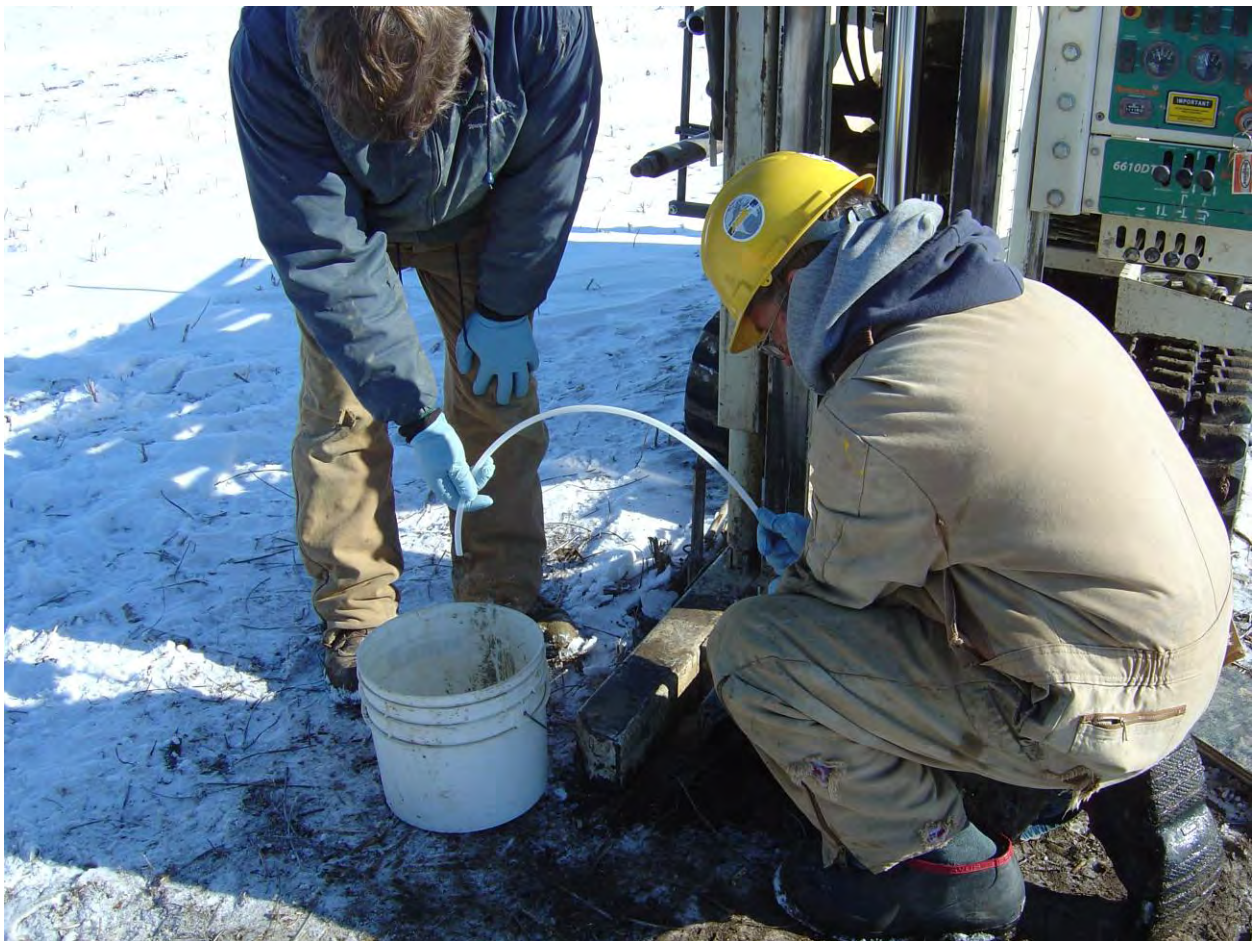
Collecting a groundwater sample using direct-push technology.
