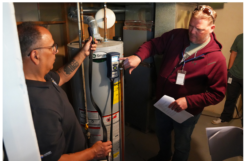
Photo courtesy United Way of the Midlands NDEE Environmental Specialist Craig Schieffer demonstrates how to use a combustion analyzer to test a water heater for efficiency and draft.
