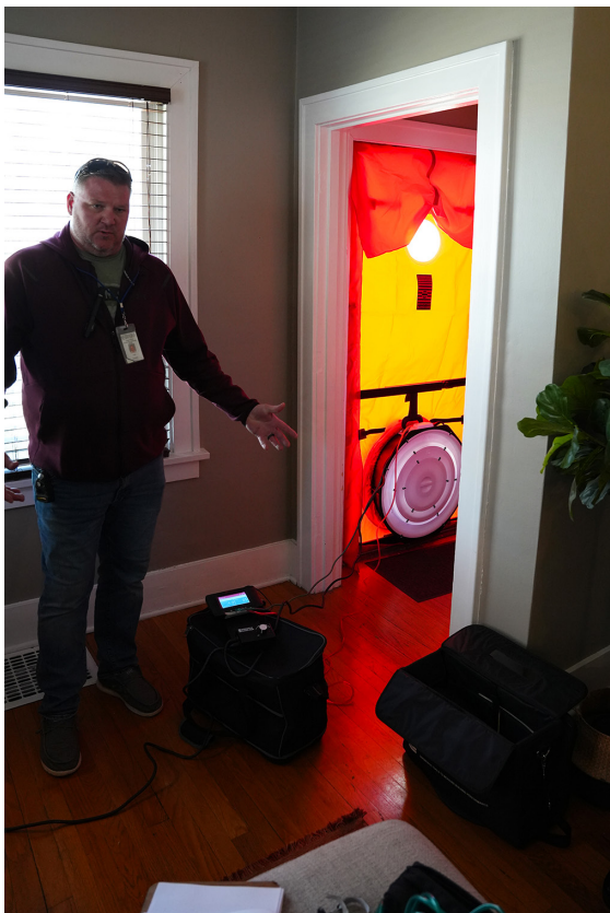
Photo courtesy United Way of the Midlands NDEE Environmental Specialist Craig Schieffer demonstrates how to run a blower door test.
