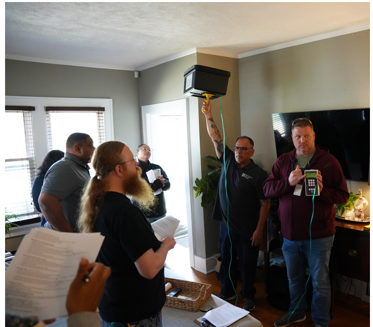
Photo courtesy United Way of the Midlands Mike Linarez, the director of the Weatherization Program at United Way of the Midlands, and Craig Schieffer, environmental specialist at NDEE, demonstrate a fan flow meter and a monometer, which measure fan flow on a kitchen or bathroom fan.
