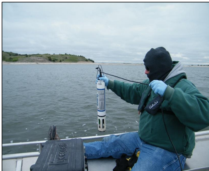
Meter used to collect depth profile data of water temperature, dissolved oxygen, conductivity, and pH, at Merritt Reservoir south of Valentine.
