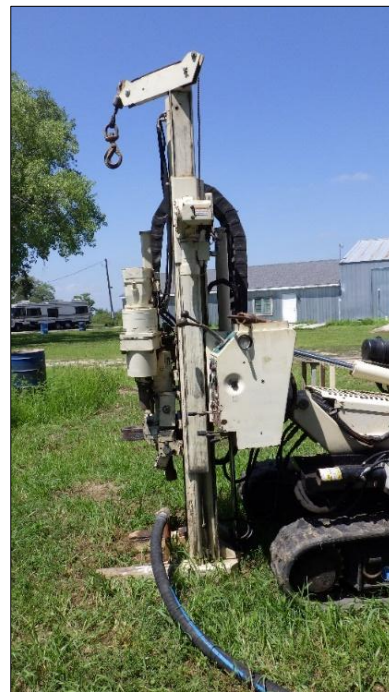
Photo shows a direct-push rig preparing for in-situ enhanced bioremediation injections into the aquifers beneath the Former Lincoln Air Force Base Atlas "F" Missile Site 1 in Elmwood, NE.
