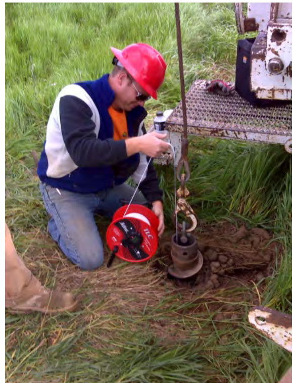
NDEQ staff measuring the water level in a test hole, Holt County
