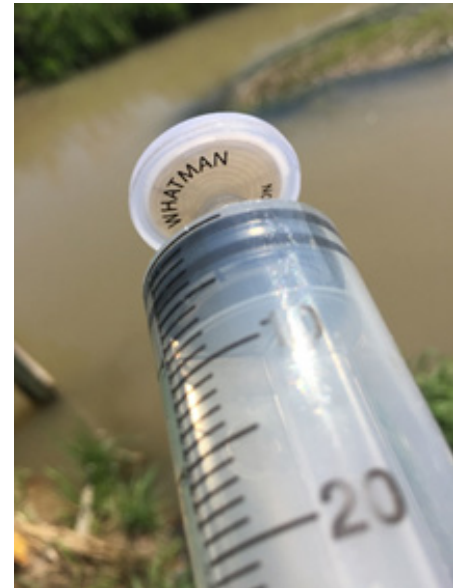
eDNA filter attached to a syringe used to determine the algal species inhabiting a stream.
