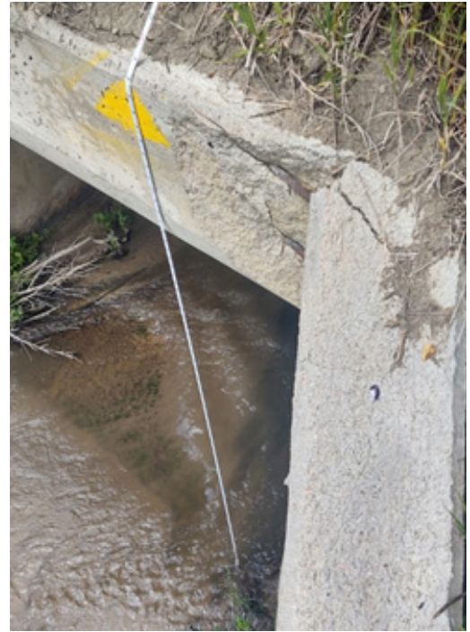
(Bottom) Measuring gage height of a stream with a weighted tape measure from a reference point marked on a concrete culvert.
