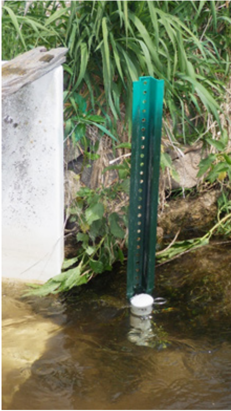
(Above) Temperature sensor deployed in the waters of East Branch Verdigre Creek, Antelope County. (Top right) Downloading temperature data from a sensor.
