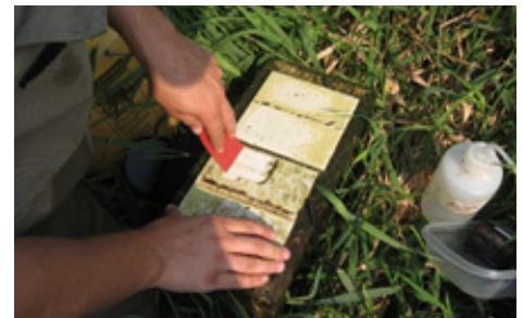
(Left) Multi-parameter meter and benthic algae tiles deployed in the water at Monroe Creek, Sioux County. (Top) Collecting samples by scraping algae colonized from benthic tiles to identify algal species and determine chlorophyll- a concentrations.
