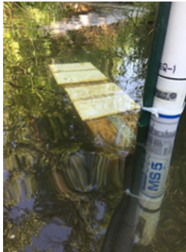
(Left) Multi-parameter meter and benthic algae tiles deployed in the water at Monroe Creek, Sioux County. (Top) Collecting samples by scraping algae colonized from benthic tiles to identify algal species and determine chlorophyll- a concentrations.
