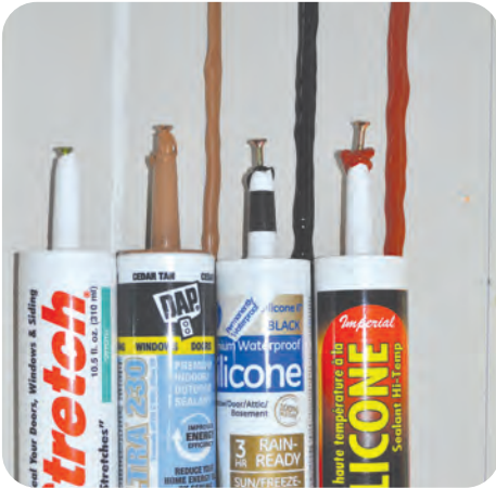
Apply caulk to areas with gap 1/4 inch or smaller
