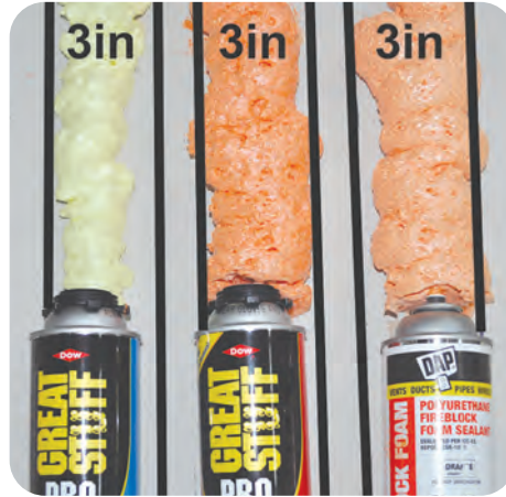
Apply sprayfoam or mastic to gaps 1/4 inch to 2 inches wide
