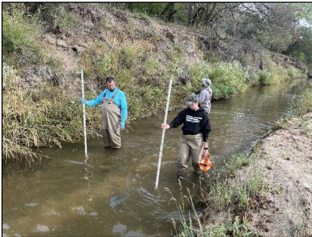
Conducting stream transect measurements
