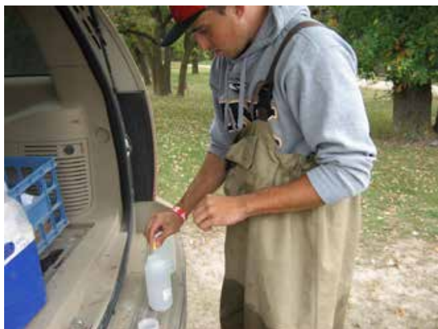
Preserving water samples collected at an ASMP site.
