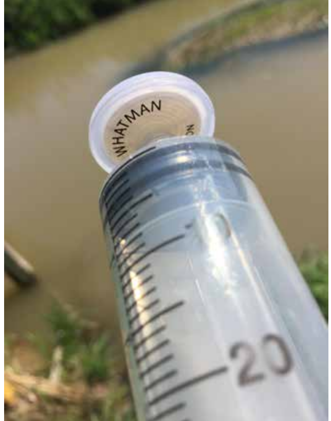
eDNA filter attached to syringe at Tub Springs Drain, Scotts Bluff County.
