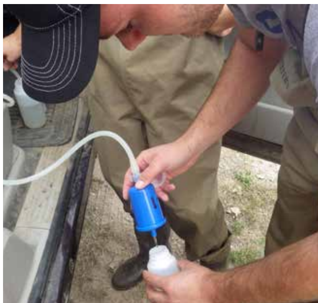
Filtering water sample to be analyzed for various heavy metals.
