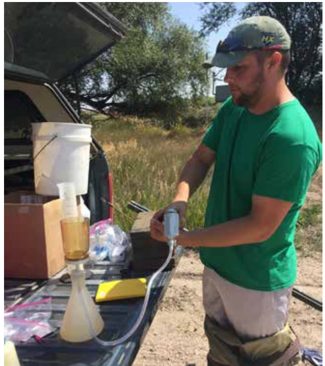
Preparing to filter a benthic chlorophyll sample collected from Tub Springs Drain, Scotts Bluff County.
