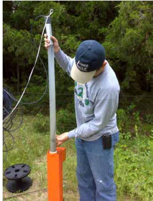
Lower Loup Natural Resources District utilizing a passive diffusion sampler to sample a monitoring well near Duncan, NE.
