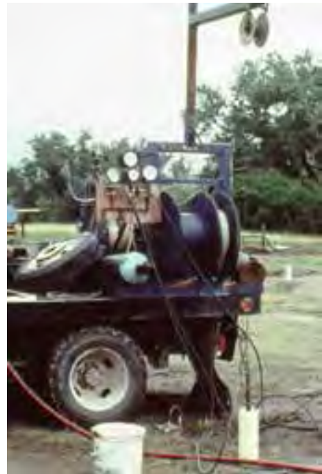
Mechanical Integrity Test at Crow Butte Resources Inc., Dawes County.
