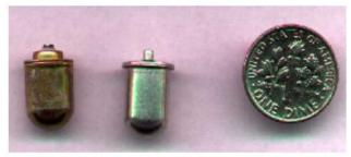
The object on the left is a mercury switch. The center object is a ball bearing switch that contains no mercury. Dime shown for size comparison.
