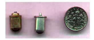
The left object is a mercury switch. The center object is a ball bearing switch with no mercury. The dime is shown for the purpose of size comparison.
