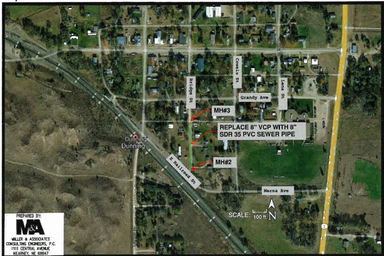
Figure 1 – Approximate Location of Village of Dunning’s Completed 8 Inch (green) Emergency Sewer Replacement
