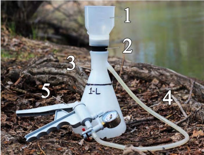
1. Filtration funnel. 2. Magnetic base with rubber stopper 3. Vacuum flask 4. Tubing 5. Hand vacuum pump with pressure gauge (Nalgene or equivalent) 2
